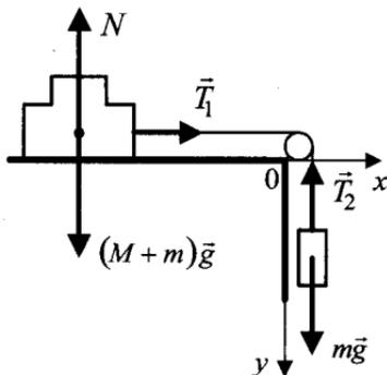
$$\left. \begin{aligned} O_x: (M+m)a_1 &= T_1 \\ O_y: ma_2 &= mg - T_2 \end{aligned} \right\}$$
